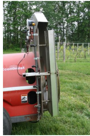
Figure 1. Cornell doughnut on air inlet Figure 2. Adjustable louvre on the air outlet
